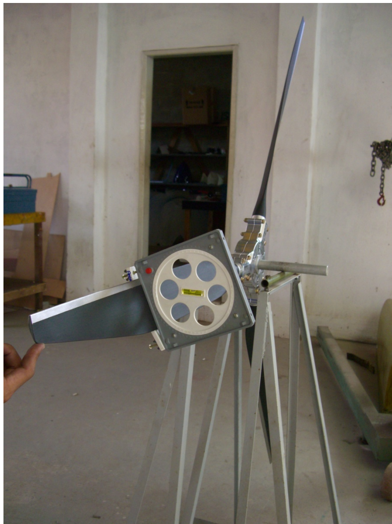
Figure 2 - Warp Drive Propeller pitch adjustment with protractor.
